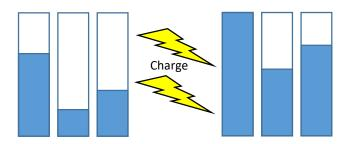
This would require draining the battery cells until all were depleted and then recharging until full to rebalance all the cells.
