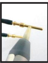
4) Apply Nyogel to the new pins and into the corresponding holes.
