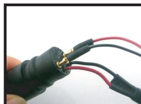
5) Position the new seat sensor pins into holes. The red wire goes in the 'D' hole and the black wire goes into the 'A' hole.
