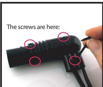
1) Locate the 4-pin rubber plug (R4) which plugs into the large plug on the front panel of the Cox-Box. The receptacle is in the shell and connects the wiring harness to the Cox-Box. Using the torx wrench, unscrew the four screws holding the plastic case in place. Gently pry the case open, and remove the R4 plug and wires from the plastic case.
