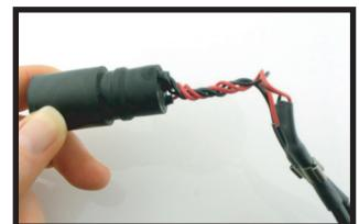
8) Twist the installed wires together.
