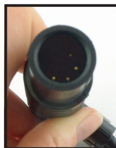
7) Check to make sure that the new pins should be even with the existing audio pins ('B' and 'C').
