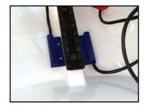
**NOTE:** Multiple sensors can be mounted around one impeller, simply mount them next to each other, or stack them on top of each other. (i.e. if you have a mounting harness in both seats of a double.)
