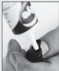
1. Apply Nyogel grease to both sockets. Be careful not to overfill, a small amount is needed.
