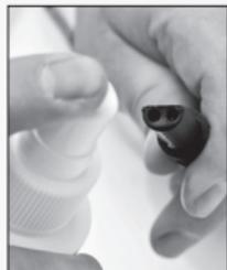
1. Use alcohol to clean the inside of the connector sockets.
